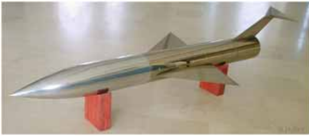
Figure 1. AGARD-C model with a body diameter of 115.8 mm
