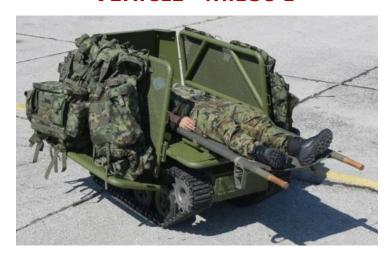
The UGV is designed to give logistic and rescue support in all possible dangerous situation in a field. It has possibility of completely wireless remote control of all function of the system through control posts in command-control vehicle or from a portable post from a remote and safe place.
