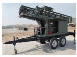
Loitering ammunition system SM-2 has been designed as a modular system of a relatively small weight. The loitering ammunition / aerial vehicle is launched from the ground, it is equipped with two-stroke internal combustion engine and it uses a global navigation satellite system (GNSS) for guidance.
