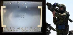
The system for operators target indication for portable air defense systems ŠILO – TRACER system is a reconnaissance device intended for surveillance and guidance of light portable rocket systems for air defense actions in order to destroy targets in air space during day and night. The system collects and processes digital data on the target, obtained by the modernized radar Giraffe, as well as by other radars according to the protocol of radar data exchange (ASTERIX).
