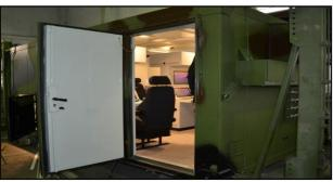
Mobile surveillance and early-warning center MCVOJ M23 enables a display of a unique radar image formed based on data from various radar sensors and superior automatization systems for the Air Surveillance, Early-Warning and Guidance Center. It conducts the reception and processing of data from all available sensors, exchange of data and information from automatization systems for the Air Surveillance, Early-Warning and Guidance Center and Fighter Aviation guidance. The system MC VOJ presents a
