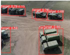
Al TARGET is an artificial intelligence model developed in the Military Technical Institute with the aim to be used in operations of the field surveillance, detection, identification and destruction of enemy targets. This model can be integrated into unmanned aerial vehicles used for the field surveillance. The model can be applied in an independent operation mode of the unmanned aerial vehicles destroying the identified targets without a pilot's command.
