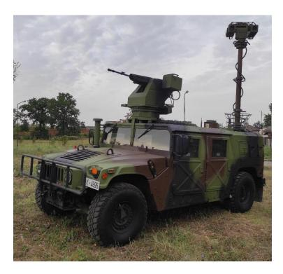
The vehicle is equipped with multisensor reconnaissance platform mounted on the telescopic mast that is integrated on the rear side of the vehicle.
