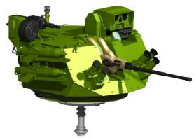
Remote controlled weapon station 20 mm is designed to be integrated on various existing and future vehicle platforms. Main purpose of the RCWS is destruction of infantry, armored and other vehicles and tanks using integrated weapons up to distance of 3.000 meters. In the case of power loss RCWS can be operated like traditional turret designs.
