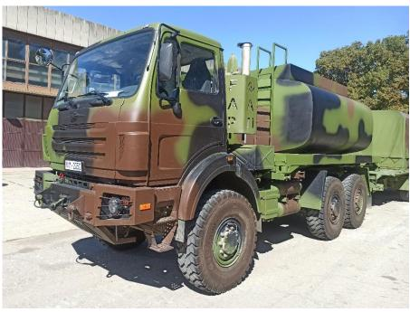
Modernized off-road vehicle FAP 2228 is intended for transport of personnel, transport of weapons and equipment with a weight of up to 7 t.
