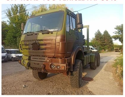
FAP 3040 BDST/AV off-road tug vehicle is intended for towing the semi-trailer with total weight of up to 41 t, as well as of a trailer with weight of up to 18 t. The vehicle is equipped with a winch for pulling of damaged and malfunctioning equipment. Also, the tug vehicle can be used for towing (with a tow bar) of damaged and malfunctioning equipment of up to 18 t weight.
