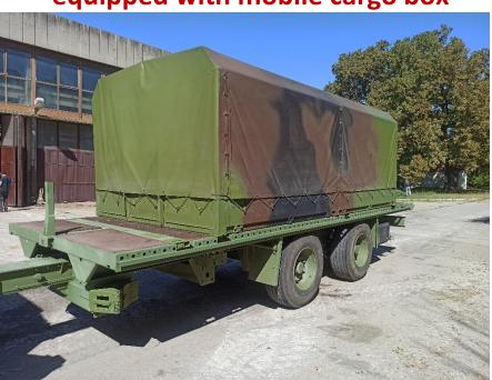
Tandem-axle trailer for container transport is intended for an integral transport, i.e. transport of containers on the field, whose weight does not exceed 14 t.
