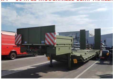
NPP-30 M 25 modernized semi-trailer is intended for transport of lightweight combat vehicles engineering systems and non-combat vehicles, whose total weight does not exceed 30 t.
