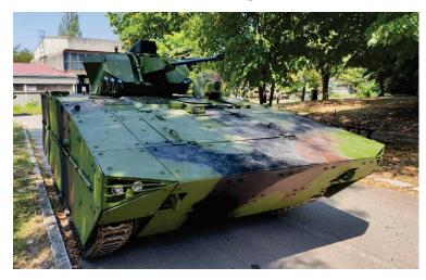
Remotely controlled weapon station of 30 mm is intended for destruction and neutralization of live force, armored and other combat systems on the ground and low-flying targets in air space, from short halts and from stationary positions at effective combat ranges of integrated weapons.
