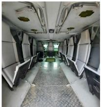
Main purpose of MRAP vehicle is to provide protected mobility of infantry soldiers and safe transport in various situations during actions, multinational operations, as well as in the high risk terrains. Driving platform has been based on FAP 2228 off-road vehicle, which helps in unification of spare parts and provides high maneuverability.
