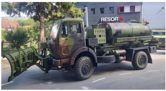
Off-road vehicle FAP 1118 is intended for transport of up to 4 t equipment on the terrain.
