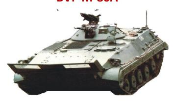
BVP M-80A is light armored, tracked, amphibious combat vehicle of the mechanized division, intended to destroy and neutralized the live force, armored and other targets on the ground and in the air at the distances of the efficient actions of formation armament and personal armament of the mechanized division, for overcoming the contaminated zones and for overcoming the water obstacles by sailing.
