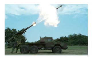
TSMB 203 mm - Heavy self-propelled mortar of 203 mm caliber is a heavy artillery short-range system, integrated on the chassis of the FAP 2026 off-road vehicle, 6x6. It is intended for destruction of fortified enemy positions.
