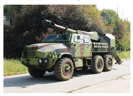
"NORA B-39" self-propelled gun howitzer 152/155 mm is intended for fire support to infantry units, destruction of enemy fortifications, neutralization of threats, high responsiveness, mobility and flexibility in various field conditions. Self-propelled gun howitzer is an essential system in contemporary military operations, enabling artillery supremacy and protection of the units in the field.
