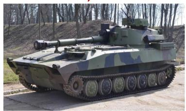
Serbian 122 mm self-propelled howitzer 2S1 "Gvozdika-Carnation", modernized, is a lightly armored artillery weapon system with a circular action, based on the automotive and running gear of the Russian MT-LB multipurpose tracked armored chassis, which enables the protection of the crew, devices and instruments from the action of small arms and pieces of artillery projectiles.
