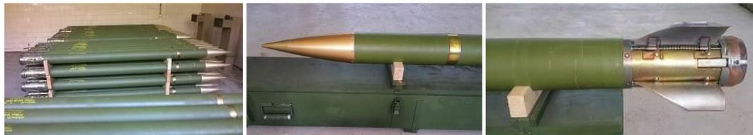
128 mm rocket with maximum range 22 km is a part of the multiple launch rocket system MLRS 128 mm OGANJ. It can be also launched from a modular multiple launching rocket system.
