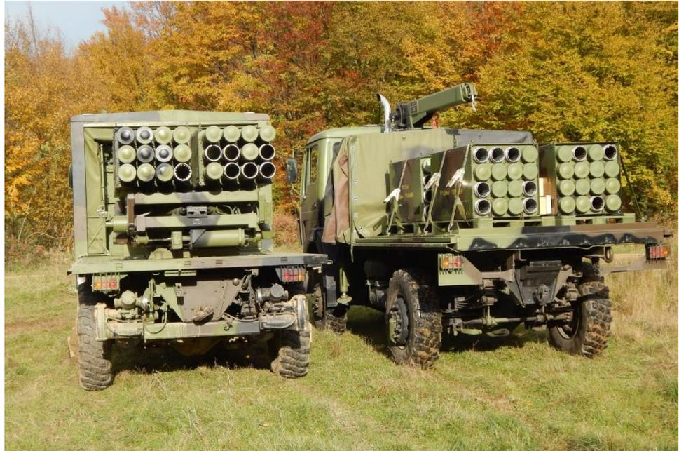
Logistic vehicle MORAVA serves to reach the army position with combat complet of modules containers. Its function is to load LRSVM "Morava" with rockets launching modules containers and to exchange used modules with new ones.
