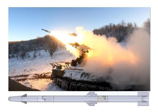
**STRELA-1MS** is a short-range air defense missile made based on improved 9M31M STRELA-1M missile, with minimum and maximum target area of 10 km, depending on the target.
