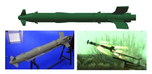
Guided missile ATGM 2T-5 is an anti-armored missile of a long range. It is equipped with over-caliber tandem shape charged warhead of increased penetration, which enables neutralization of tanks and other armored vehicles, with or without ERA, as well as for neutralization of firing posts and fortifications, at the distances from 750 m to 5.000 m.
