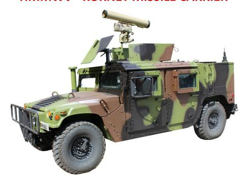
The vehicle is equipped with basic armor and a Kornet anti-tank missile launcher mounted on the roof of the vehicle. The vehicle is used for transport and launch of a Kornet anti-tank missiles as primary weapon system with possibility of having PKT 7.62mm machine gun as secondary weapon. The weapons platform could be traversed 360 degrees.
