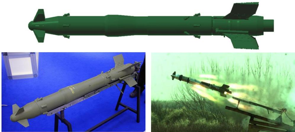
Guided missile POVR 2T5 is an anti-armored missile of a long range. It is equipped with over-caliber tandem shape charged warhead of increased penetration, which enables neutralization of tanks and other armored vehicles, with or without ERA, as well as for neutralization of firing posts and fortifications, at the distances from 750 m to 5.000 m.
