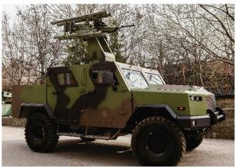
The MTU-4M system obtains receiving and processing of target data from radar "Giraffe". Digital data processing includes correction of received target data depending on the radio signal delay from the radar, prediction by linear tracking, calculation of the distance to the target and target azimuth.
