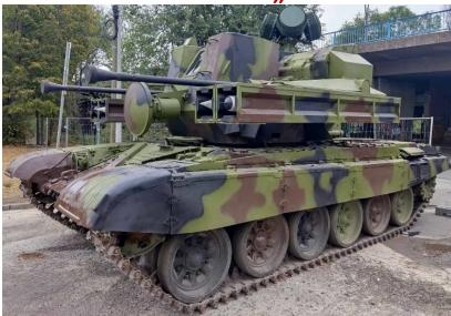
"HARPAS" system is a modern hybrid artillery weapon system intended for anti-aircraft defense of troops and important objects from airplanes, helicopters, cruise missiles and unmanned aerial vehicles. It is integrated on the vehicle base of the M84 main battle tank, which is characterized by excellent mobility and the ability to protect the crew, devices and instruments from the action of small arms and pieces of artillery projectiles.
