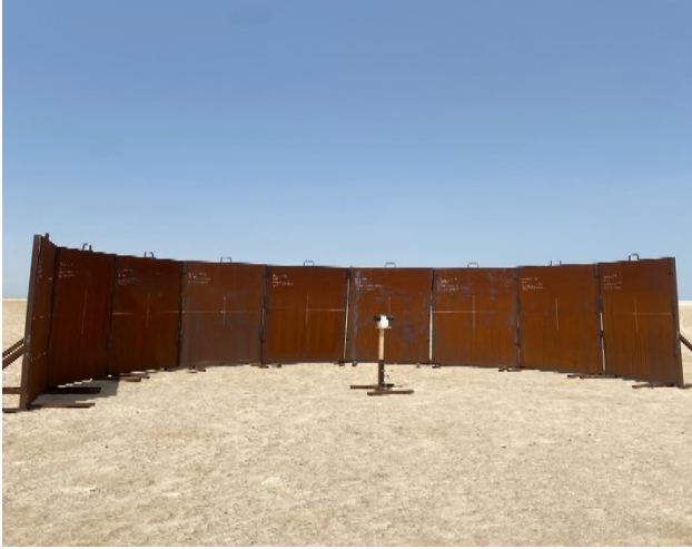
Figure 11. Horizontal Arena Test Setup.
