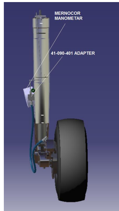
Figure 3a. Pressure gauge installation
