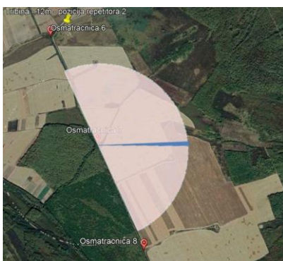
Figure 4. Coverage area with vMSIS3-USD2-C225 in patrol mode of operation
