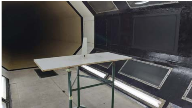
Figure 5 Wind tunnel flutter test setup
