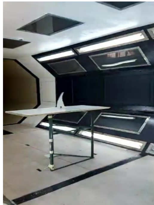
Figure 6 wind tunnel flutter test
