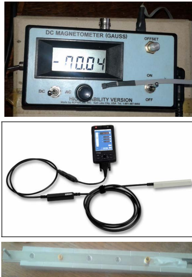
Figure 8. Equipment for testing homogeneity of the magnetic field, magnetometers: a) “AlphaLab Inc.” and b) “Metrolab” and c) slider with brake
