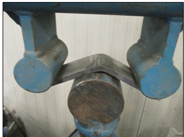
Figure 4. Root bend test.
