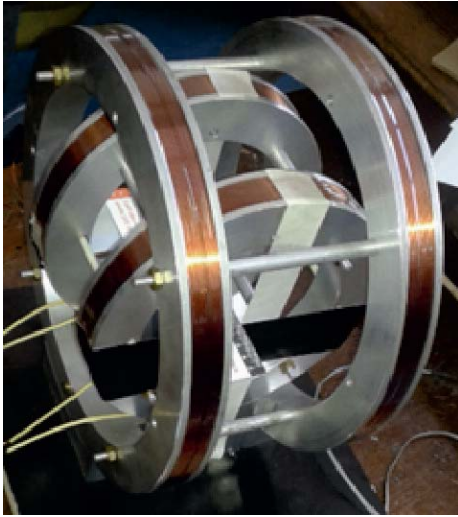
Figure 12. Arranging coils for testing the magnetocrystalline anisotropy of the magnetic element.
