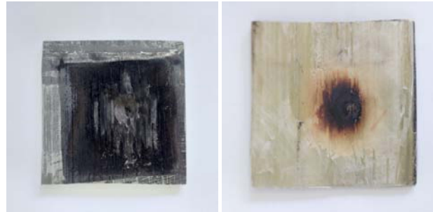
Figure 7. Samples of cured composite after ablation test
