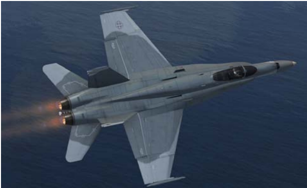
Figure 2. Strakes on F/A-18C (picture @ I. Kostić)
