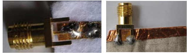
Figure 6: SMA connectors details above and below.
