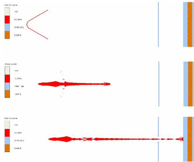
Figure 4. Jet formation process without obstacles
