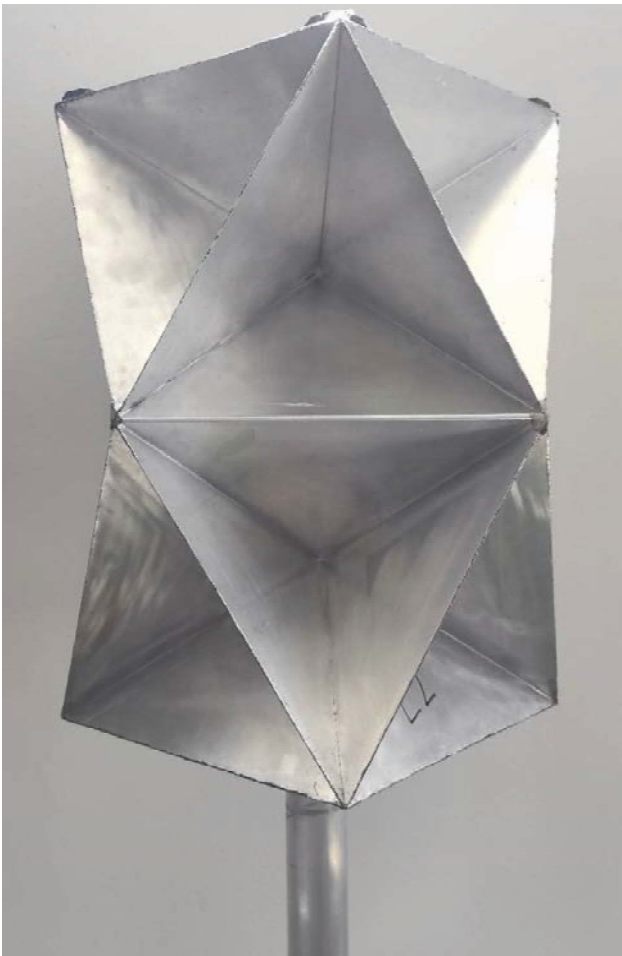
Figure 6. Corner reflector used for calibration
