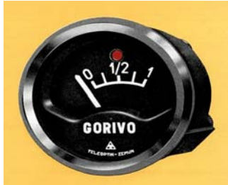
Figure 7. Type 404 fuel gauge
