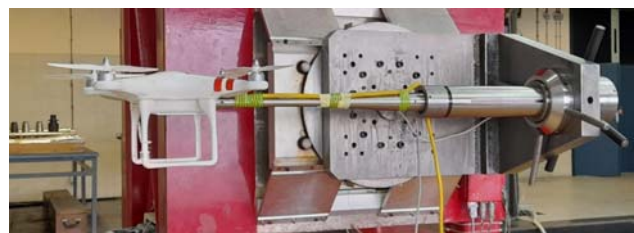
Figure 6. DJI Phantom model on the calibration rig
