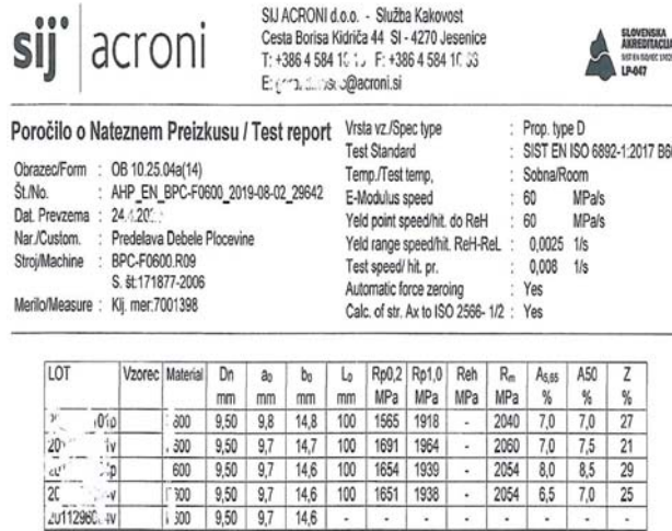
Figure 6. Results of tensile test
