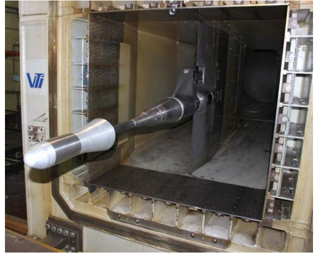
Figure 2. The 100 mm dia. HB-2 standard model in the VTI T-38 wind tunnel
