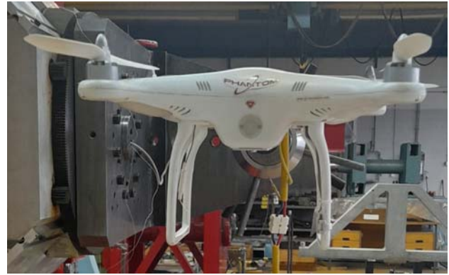
Figure 4. DJI Phantom model in the T-38 wind tunnel calibration laboratory
