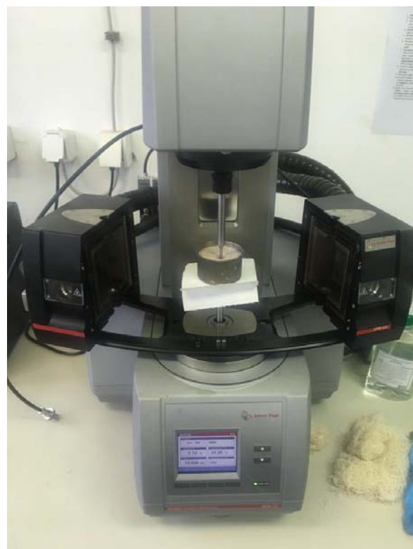
Figure 1. Rheometer MCR 302, PE adhesion and penetration resistance test
