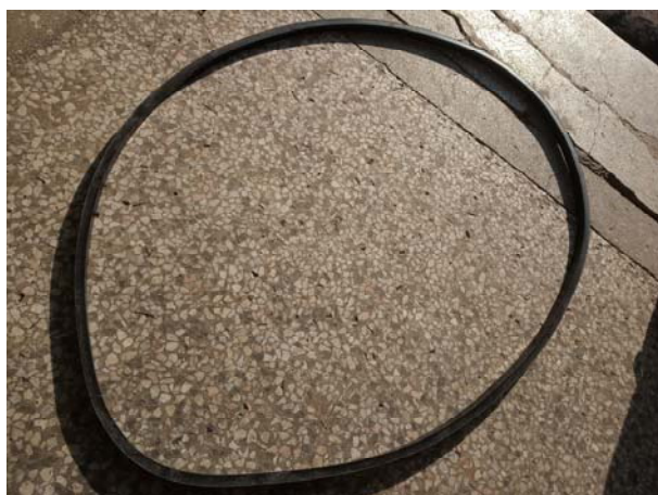
Figure 2. O-ring made of polychloroprene
