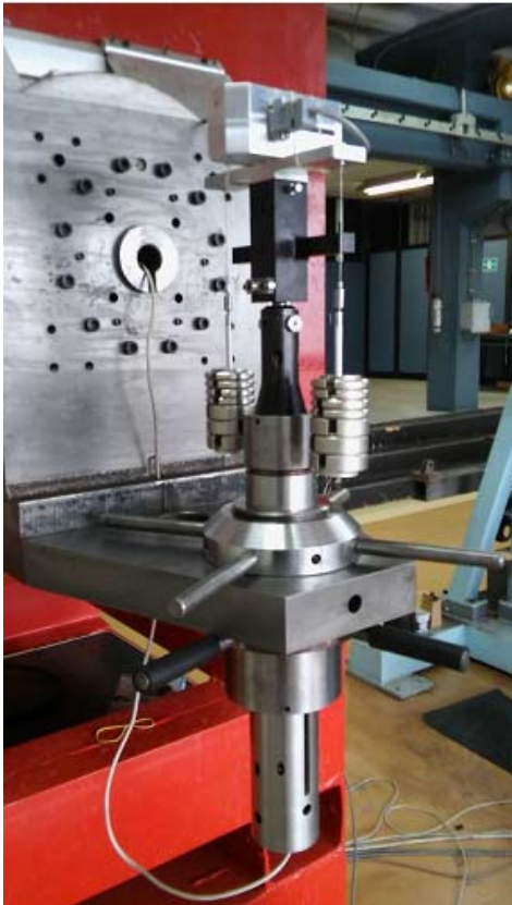
Figure 3. The six-component balance on the T-38 calibration rig
