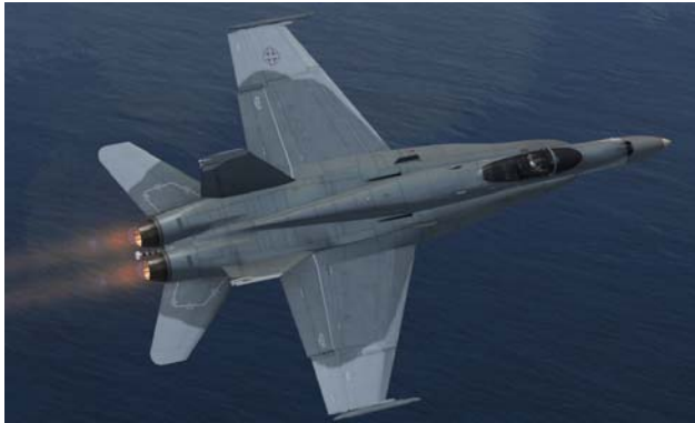
Figure 2. Strakes on F/A-18C (picture @ I. Kostić)
