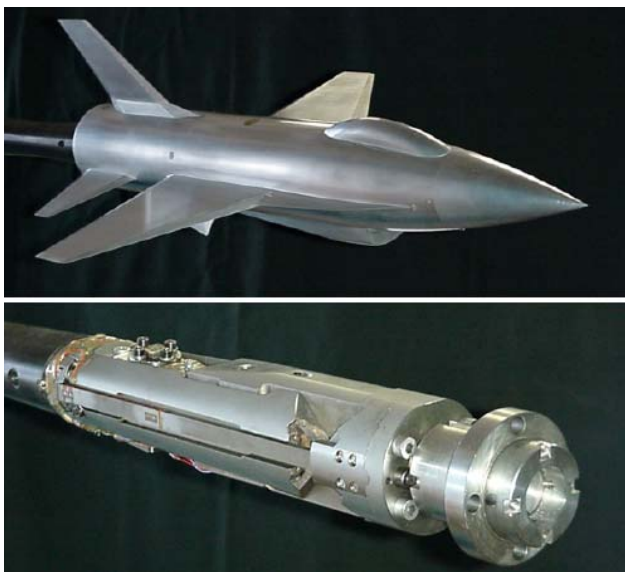
Figure 3. SDM model and pitch/yaw apparatus for wind tunnel calibrations in VTI (photo @ VTI)
