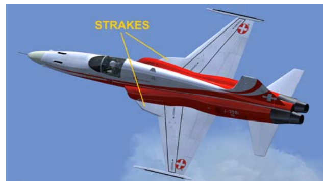
Figure 1. Double wedge strakes on Northrop F-5E (picture @ I. Kostić)
