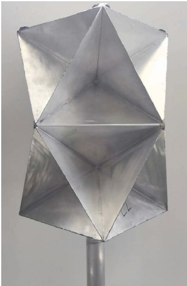
Figure 6. Corner reflector used for calibration
