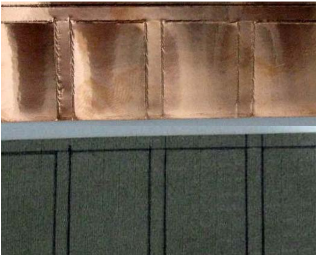
Figure 2. Copper tape and conductive textiles cut with a precision scalper [12].
