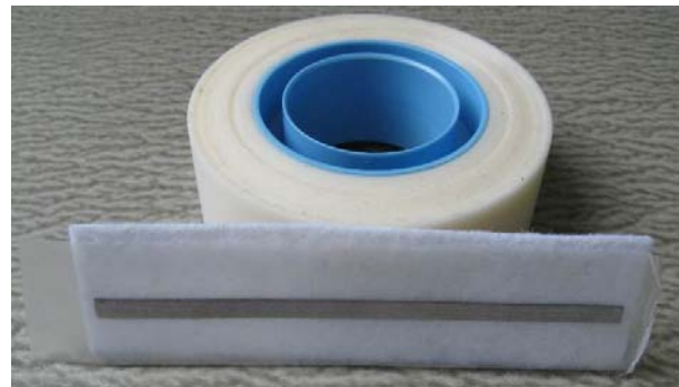
b) The supporting white paper was removed and the entire construction was glued to the substrate (felt). One can see the glued conductive textile and the self-adhesive transparent tape glued to it.
