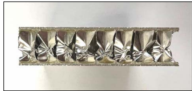
Figure 7. Appearance of the specimen after flatwise compression testing
