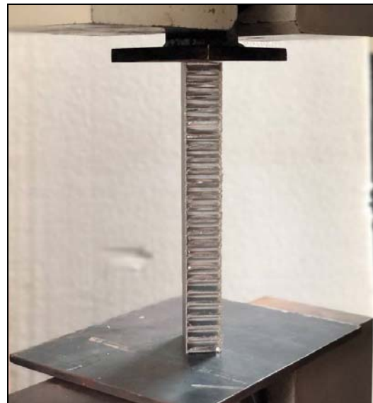
Figure 8. Sample before edgewise compressive test
