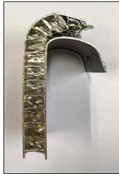
Figure 10. Appearance of the specimen after flatwise compression testing
