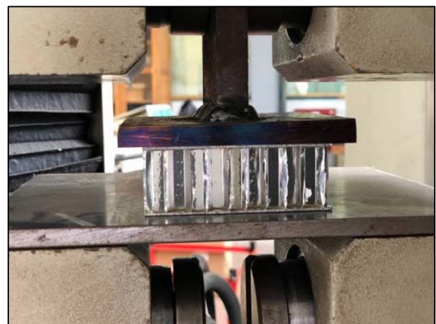
Figure 5. Sample during the flatwise compression test
