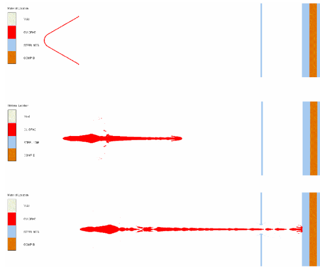
Figure 4. Jet formation process without obstacles
