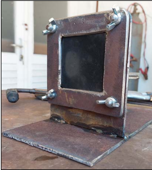
Figure 2. Specimen-fixing unit for oxy-acetylene torch test
