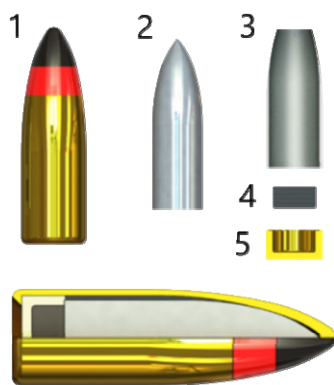
Figure 1. 7.62x39 mm API M 82 projectile: 1 – Jacket, 2 – Steel core, 3 – Lead-Antimony filler, 4 – Incendiary mixture, 5 – Tombac cup
