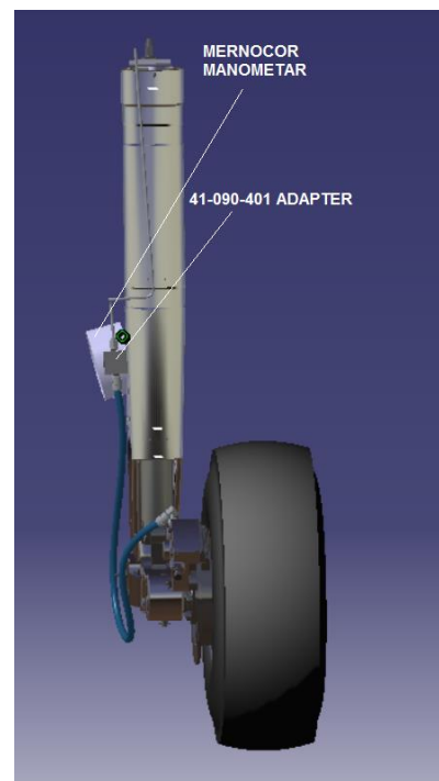
Figure 3a. Pressure gauge installation
