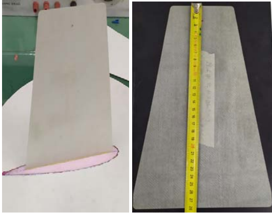
Figure 4 E-glass tapered plate for wind tunnel flutter test
