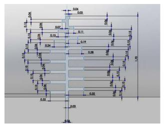
**Figure 1.** Constructive drawing of dimensioned herringbone (all measurements are given in micrometers)
