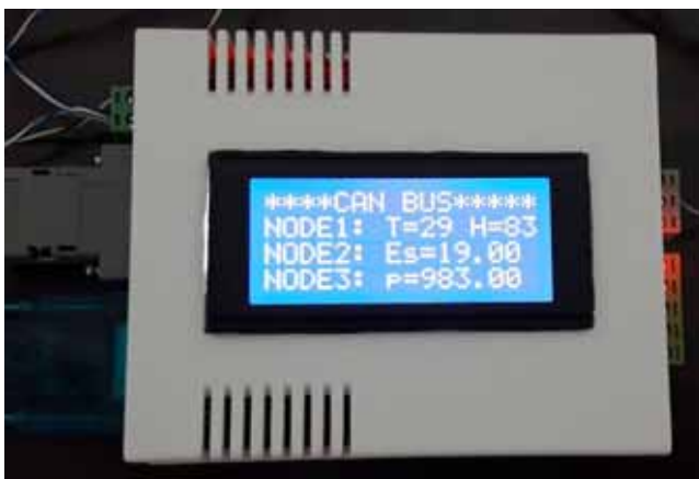
Figure 14. The values from the sensors on the testing node's LCD screen
