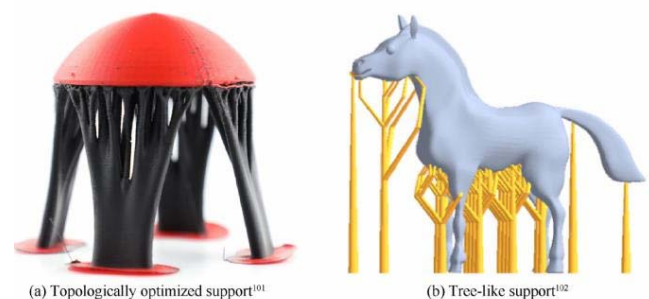
Figure 5. Innovative support design, topologically optimized support (left) and tree-like support (right) [28].
