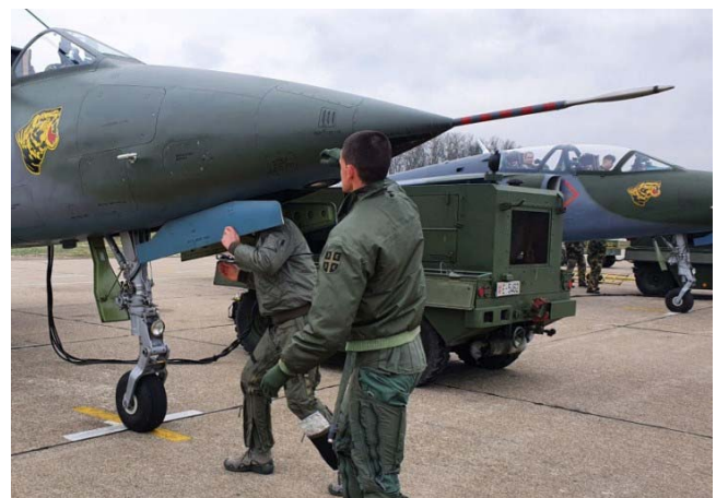
Figure 2. Pitot tube on ORAO J-22 aircraft
