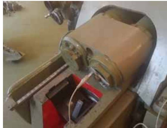
Figure 4. Installation of the two sensors (left sensor WA300, right sensor B12)
