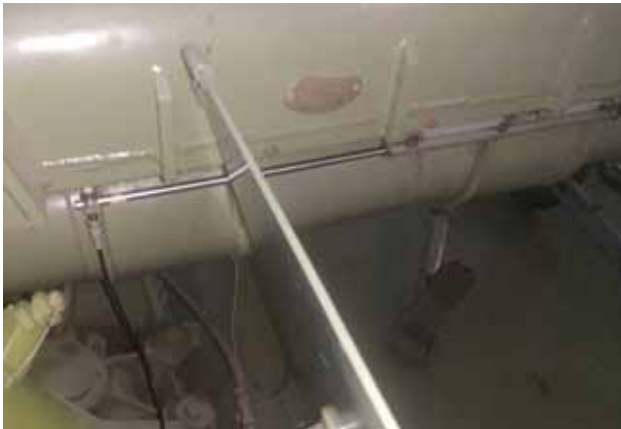
Figure 4. Installation of the two sensors (left sensor WA300, right sensor B12)
