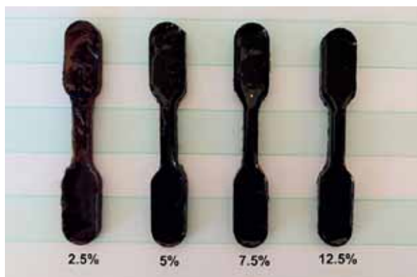
Figure 3. Standard test molds for uniaxial tensile measurements
