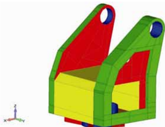
Figure 4. Display of the model of the middle surfaces of the structure of the upper carriage in the software package FEMAP.
