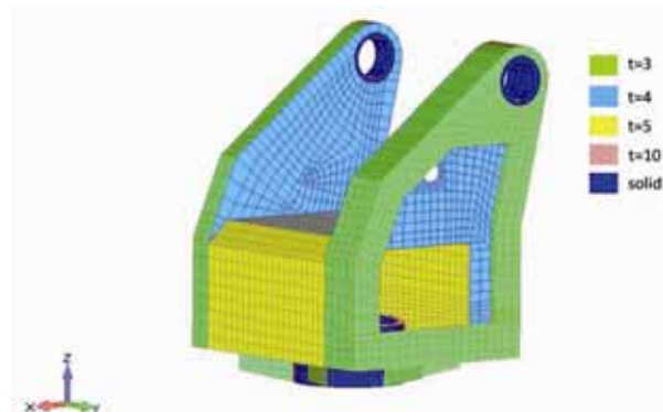
Figure 5. MKE upper carriage construction model
