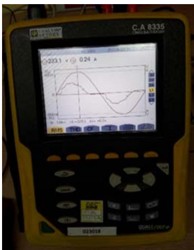
Figure 8. High precision power and quality analyzer Chauvin Arnoux C.A 8335
