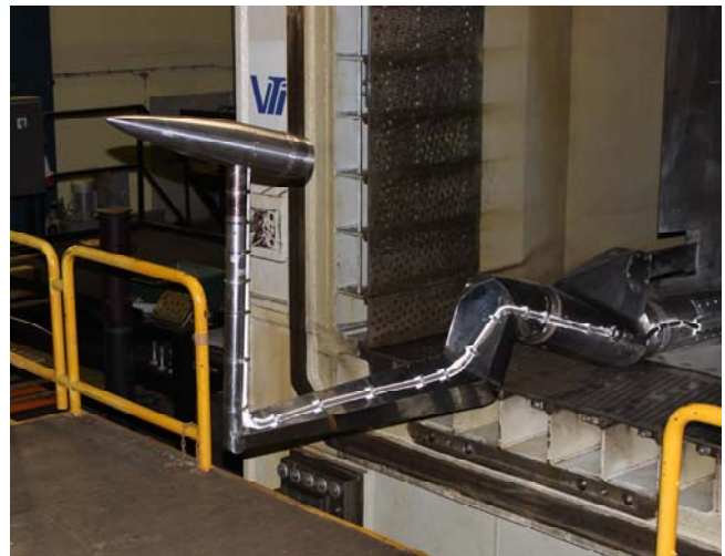
Figure 4. Model of the projectile on the 71° bent sting in the T-38 wind tunnel test section.
