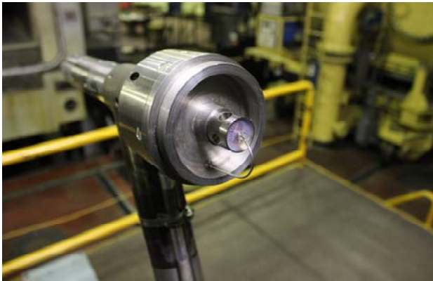
Figure 8. Pressurized-air manifold with formed temperature transducer
