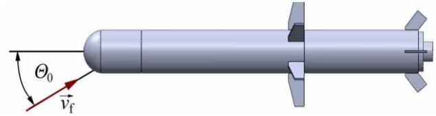
Figure 3. Interception angle between fragments and a missile
