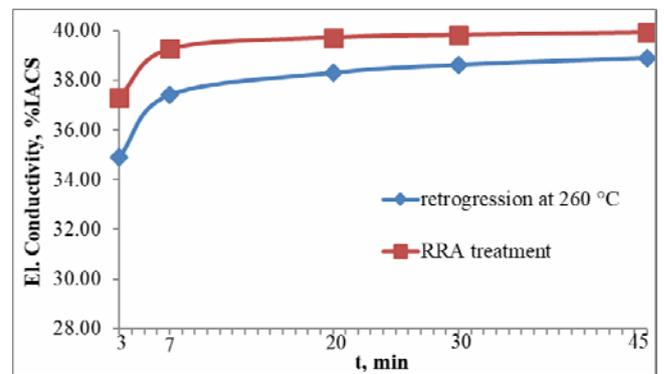
**Figure 6.** Electrical conductivity changing as a function of different holding time at the temperature of the retrogression of 260 °C.
