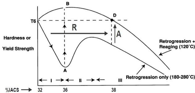
Figure 1. Schematic presentation of stages in the RRA, [3].
