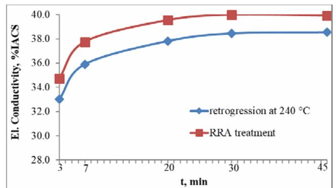
**Figure 5.** Electrical conductivity changing as a function of different holding time at the temperature of the retrogression of 240 °C.
