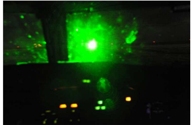
Figure 9. The intensity of the incident beam perceived from the cockpit at a distance of about 2,900 m
