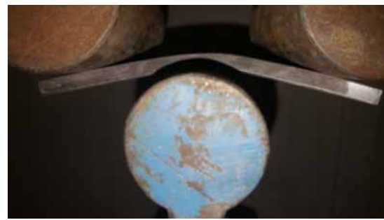
Figure 8. Three-point bending test
