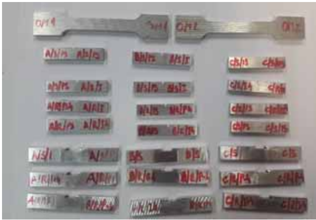
Figure 5. Tensile specimens, impact test specimens and SENB specimens
